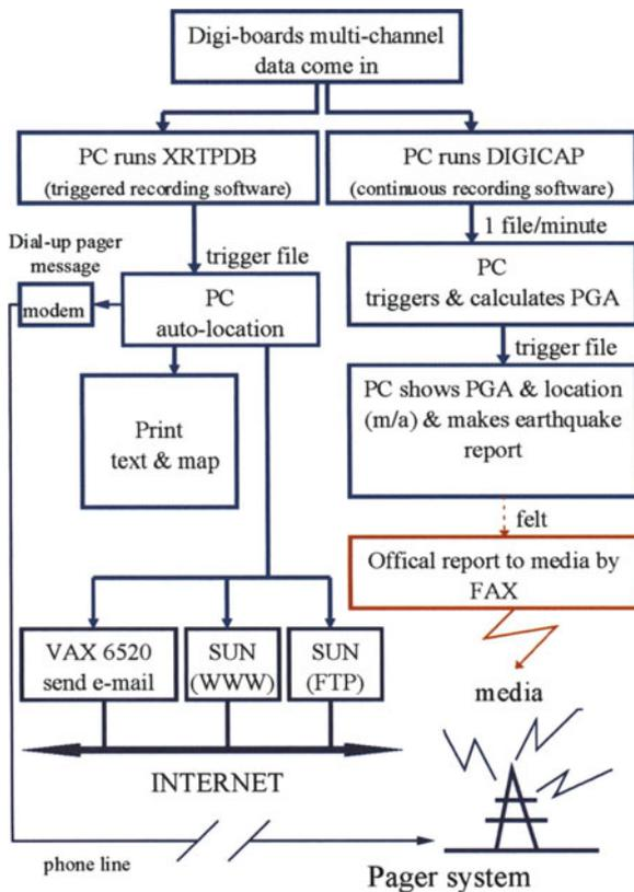
Fig. 3. A flow chart showing the data processing of the TREIRS
