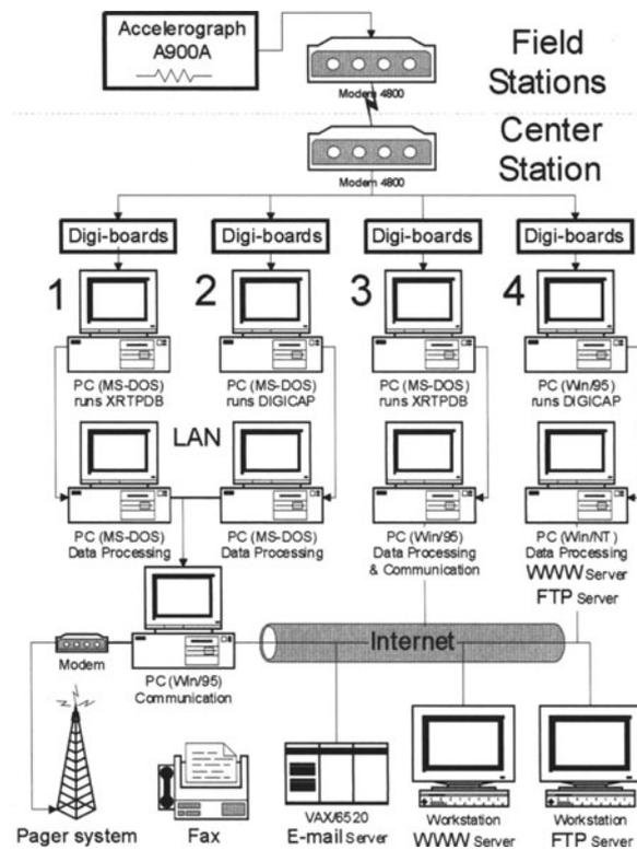
**Fig. 2.** A block diagram showing the hardware of the Taiwan Rapid Earthquake Information Release System (TREIRS)
