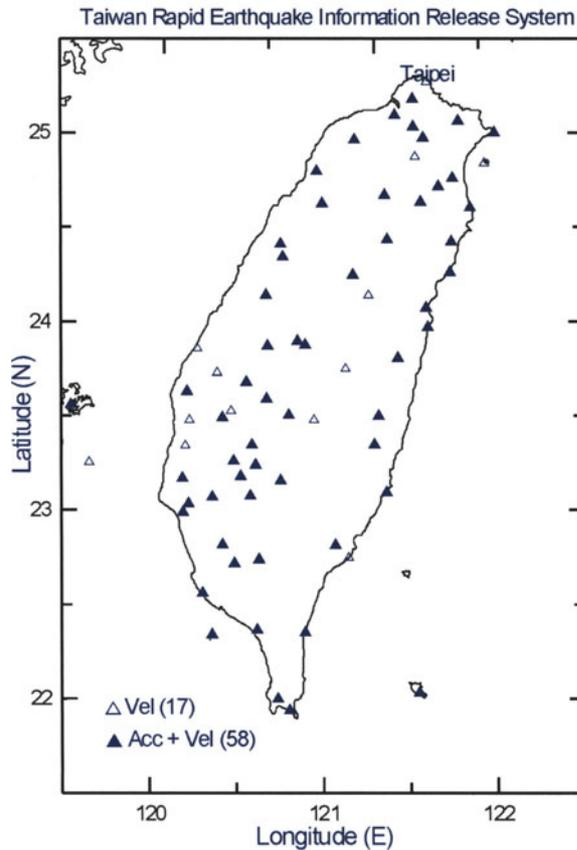
**Fig. 1.** Map showing station locations of telemetered digital accelerographs and short-period seismographs (solid squares), and telemetered digital short-period seismographs (open squares) in Taiwan
