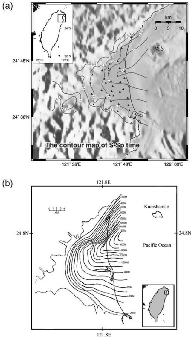
**Figure 3.** (a) Spatial distribution of the observed time differences of  $S - Sp$  arrivals. The triangles show the 44 TSMIP stations contributing to the spatial distribution. The time differences are in units of seconds. (b) The contour of thickness for the Quaternary alluvial sediments in Lan-Yang Plain. The contour map is modified from Chiang (1976). The contours are in units of meters.
