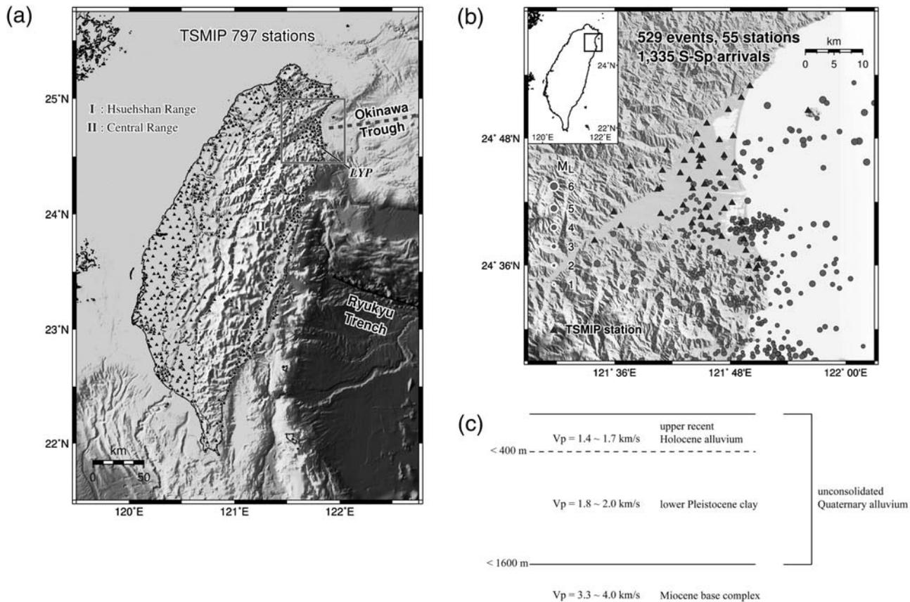
**Figure 1.** (a) Map showing a dense coverage of the TSMIP stations throughout the island of Taiwan. The Okinawa Trough is located northeast of the Lan-Yang Plain. The square (top right) includes the study area, Lan-Yang Plain (LYP), which is enlarged in (b). (b) Locations of the TSMIP stations and seismic events used in this study are shown by the solid triangles and circles, respectively. (c) Illustrative sketch of the  $P$ -wave velocity structure of Lan-Yang Plain.
