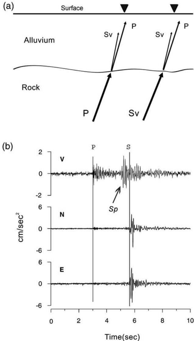
**Figure 2.** (a) Simple illustration of  $P$ - $S$  converted phases and (b) example of a typical  $S$ -to- $P$  converted phase ( $S_p$ ) recorded at an TSMIP station within Lan-Yang Plain from a local earthquake.
