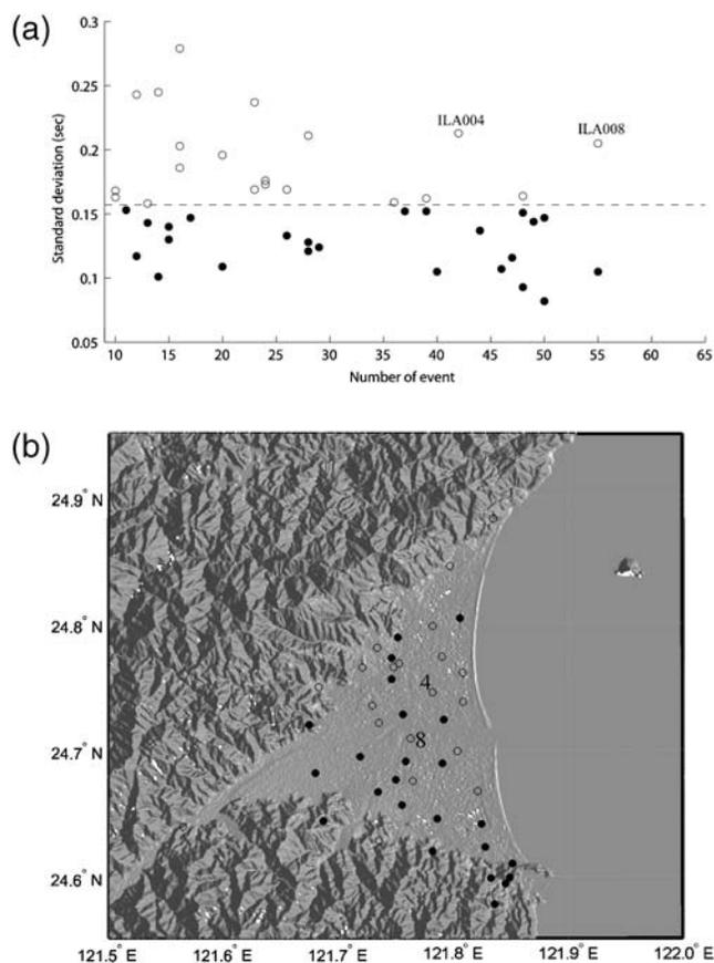
**Figure 5.** (a) Relation between the standard deviation and the number of events recorded. The dashed line indicates the average of the standard deviation. Solid and open circles represent smaller and larger standard deviations than the average, respectively. (b) Spatial distribution of the standard deviation. Numbers 4 and 8 represent TSMIP stations ILA004 and ILA008, respectively. Solid and open circles have the same representation as in (a).
