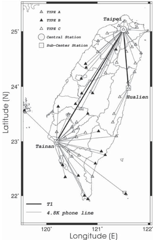
▲ **Figure 1.** Distribution of real-time strong-motion stations of CWB. Station signals during the Chi-Chi earthquake occurrence are classified A, B, or C for normal; capable to be used by the *P*-wave method; and unacceptable for analysis, respectively.
