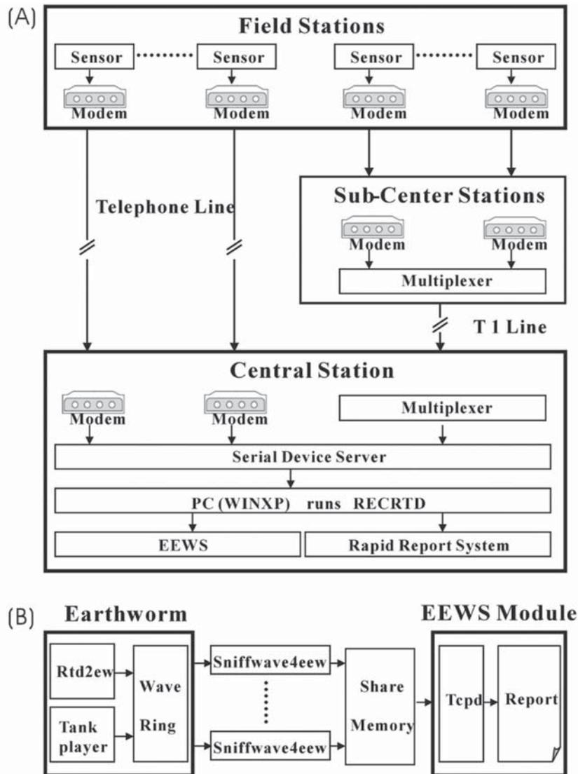
▲ **Figure 3.** (A) Hardware and (B) software configurations of the CWB *P*-wave earthquake early warning system.
