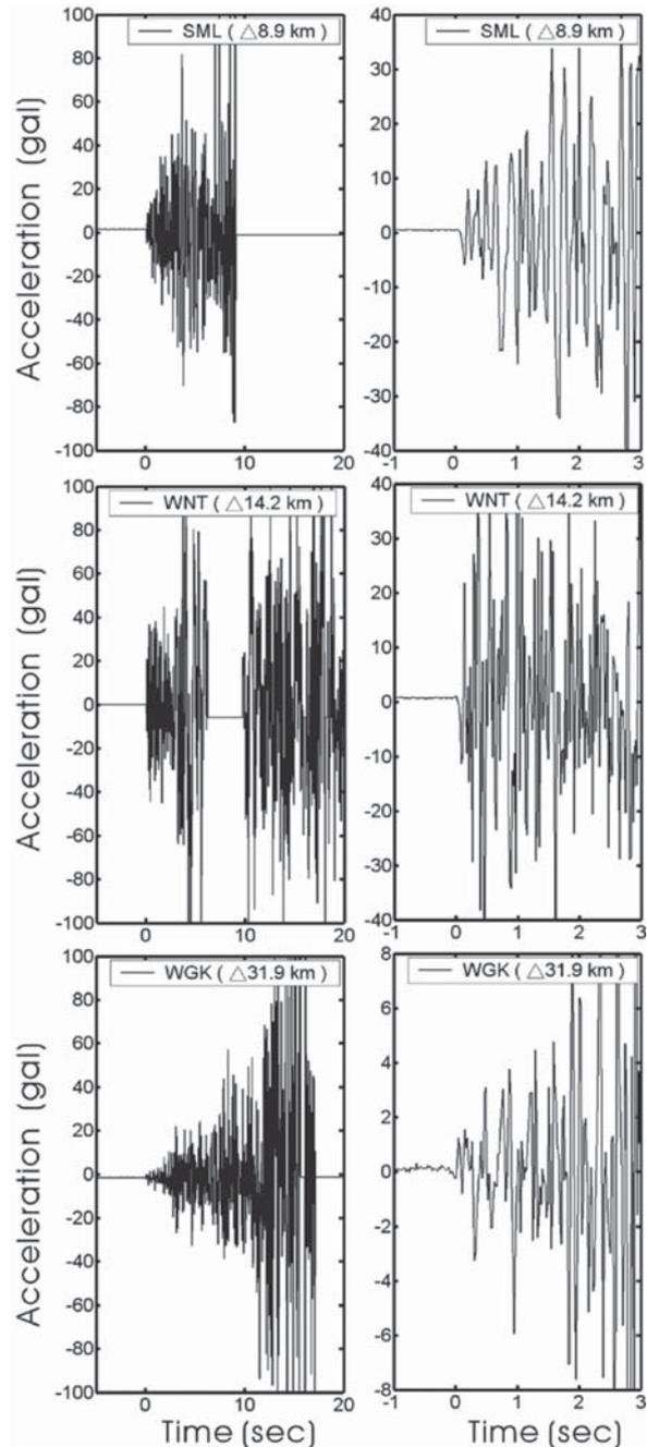
▲ **Figure 2.** The seismograms on the left show the type B real-time strong-motion signals of the 1999 Chi-Chi earthquake. The plots on the right show the initial three seconds of signals after the *P* arrival.
