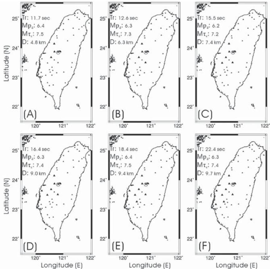
▲ **Figure 4.** Simulation results for six stages after the earthquake occurrence. Open circles and stars indicate the epicenter of the Chi-Chi earthquake from the CWB catalog and simulations, respectively. Large triangles indicate the stations (types A and B) used in simulations. Tr is the reporting time after the earthquake occurrence, and D is the focal depth from simulations.  $M_{p_d}$  and  $M_{\tau_c}$  represent the Pd magnitude and  $\tau_c$  magnitude, respectively.
