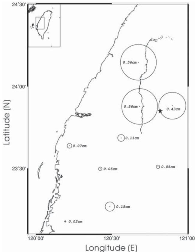
▲ **Figure 5.**  $Pd$  values of the Chi-Chi earthquake estimated from real-time strong-motion signals.
