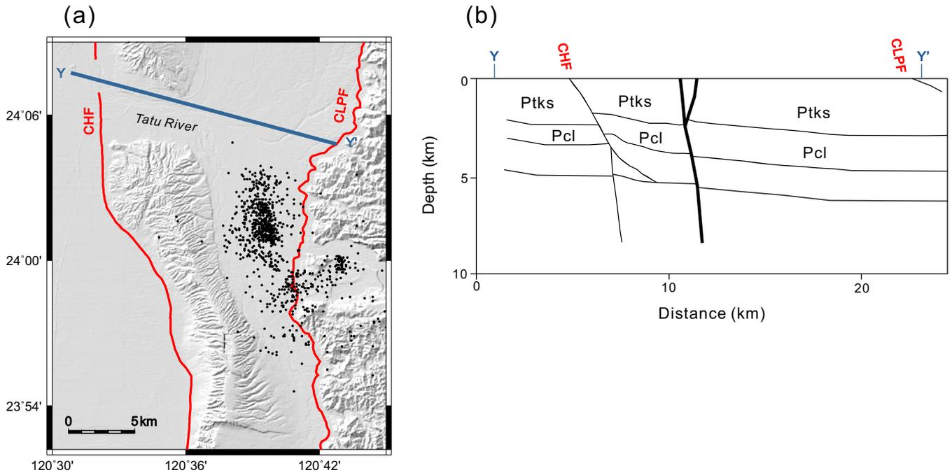
**Figure 6.** A pre-existing subsurface normal fault (shown as bold black line) is found in the footwall block of the Chelungpu fault, about midway between the fault and the Changhua fault, along an E–W seismic reflection profile (Y–Y'). Modified from line 6 of Yang *et al.* (2007). CLPF, the Chelungpu fault; CHF, the Changhua fault; Ptk, Pleistocene Toukoshan Formation; Pcl, Plio-Pleistocene Cholan Formation.
