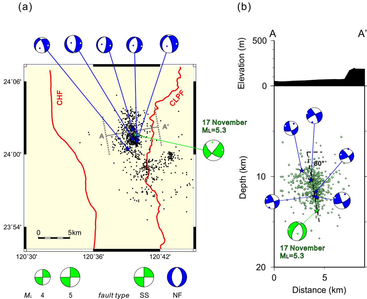
**Figure 4.** (a) Map view of the earthquake distribution of Sequence A, with focal mechanisms of events greater than  $M_4$ . (b) A seismicity cross-section along A–A', and the geometry of the proposed subsurface normal fault. Blue colour indicates normal faulting mechanism and green colour indicates strike-slip mechanism. CLPF, the Chelungpu fault; CHF, the Changhua fault.
