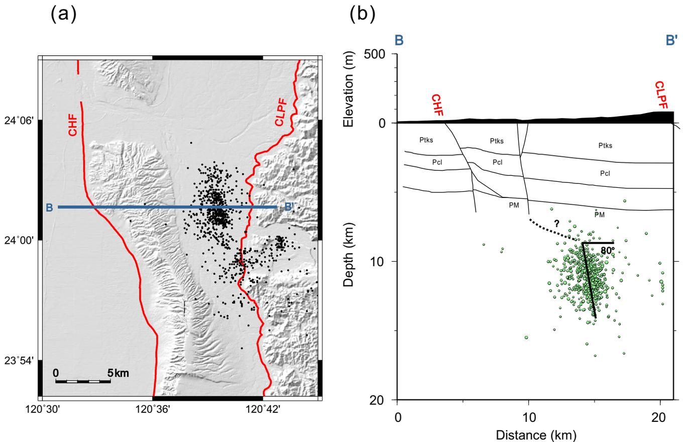
**Figure 7.** A combined projection of the seismicity profile with the seismic reflection profile along B–B' suggests that the proposed subsurface normal fault that may produce the aftershocks of Sequence A can connect approximately with the high-angle fault mapped along the seismic reflection profile. CLPF, the Chelungpu fault; CHF, the Changhua fault; Ptk, Pleistocene Toukoshan Formation; Pcl, Plio-Pleistocene Cholan Formation; PM, Pre-Miocene basement.
