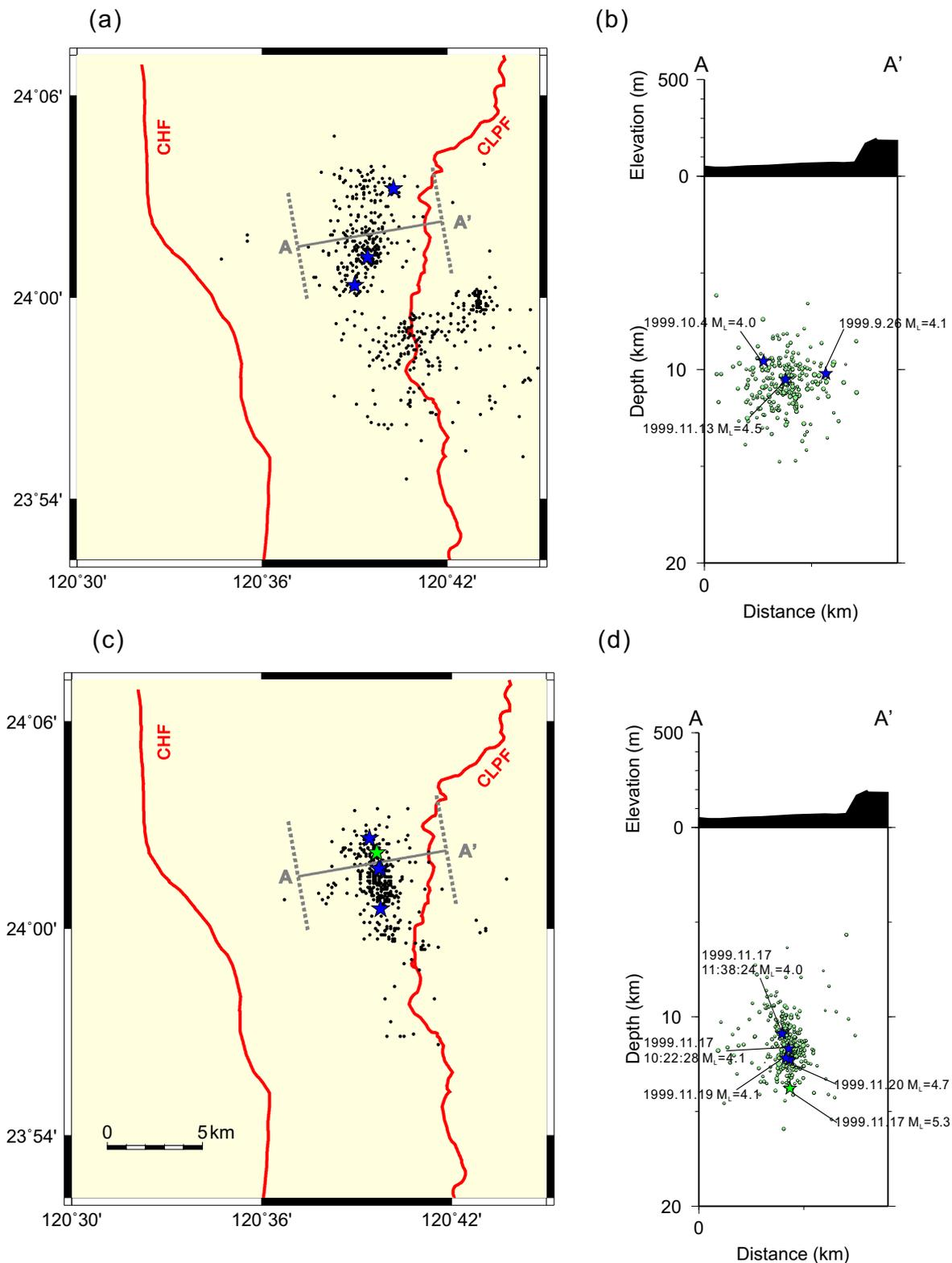
**Figure 5.** (a) Map view and (b) cross-section of the seismicity distribution before the  $M_{5.3}$  earthquake on 1999 November 17, and (c) map view and (d) cross-section of the seismicity distribution after the earthquake. Blue colour indicates normal faulting mechanism, and green colour indicates strike-slip mechanism. CLPF, the Chelungpu fault; CHF, the Changhua fault.
