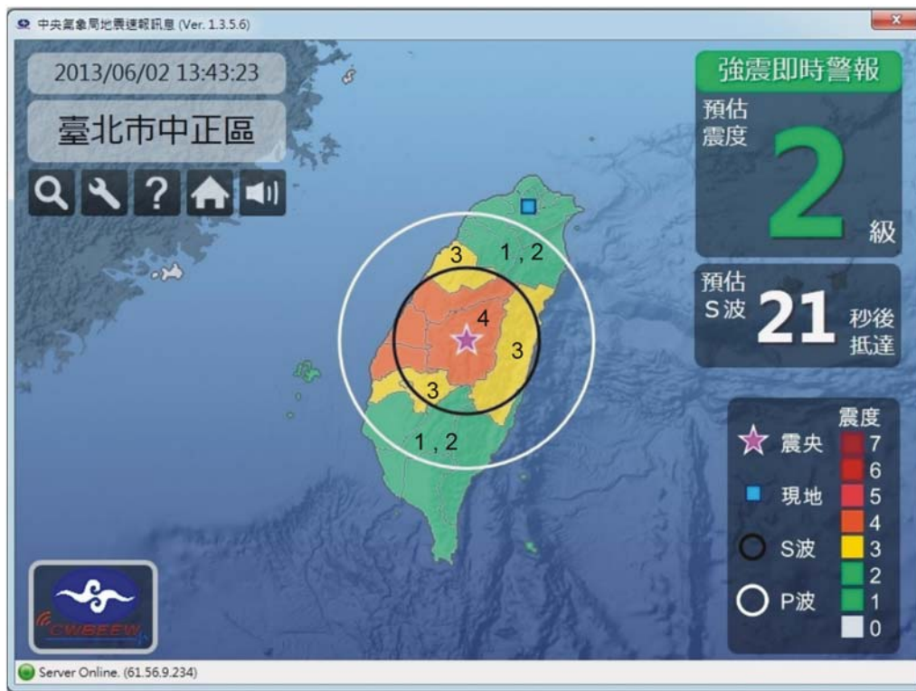
Figure 4. Graphical output of the e BEAR system during a simulation of the M_L 6.5 earthquake in central Taiwan. (top left) The origin event time and the name of the target city. (center) The square represents the target area, the black line represents the wavefront of the P wave, and the white line represents the wavefront of the S wave. (center right) The countdown timer for the S -wave arrival. (top right) The predicted intensity in the target area. The color version of this figure is available only in the electronic edition.
