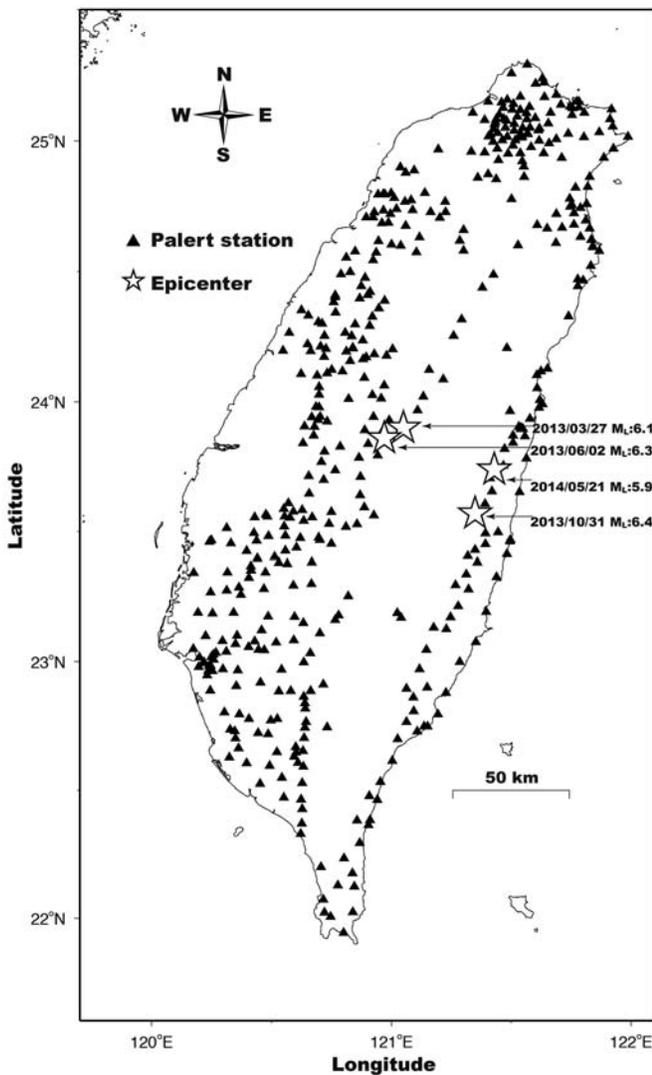
▲ **Figure 1.** Station distribution of the  $P$ -alert earthquake early warning system (solid triangles). The open stars indicate the earthquakes used in this study.
