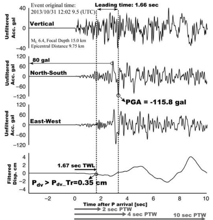
▲ **Figure 2.** Raw three-component accelerograms and 0.075 Hz high-pass filtered vertical displacement seismogram. The dashed vertical lines indicate the time points of  $P_{dv} > P_{dv\_Tr} = 0.35$  cm and peak ground acceleration, respectively.
