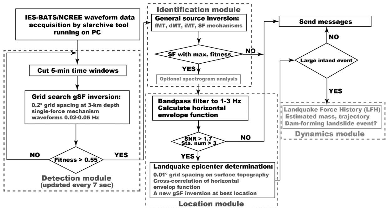
**Figure 1.** Flowchart of near real-time landslide monitoring system (NRLMS). The system consists of modules for landquake detection, identification, location and dynamics estimation. Optional procedures (spectrogram analysis and dynamics module) marked by the light grey colors are not implemented in the automatic system.
